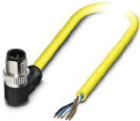
Sensor/Actuator cable, 5-position, PVC, Yellow RAL 1021, Plug angled M12-SPEEDCON, A-coded, on Free cable end, Cable length: 2 m
